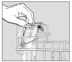
To make room for tall glasses, raise the rack upwards. Lower it to double stack smaller items.
